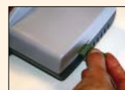
1. Turn on LifeAssays Reader and insert the disposable algorithm chip provided with test kit.
